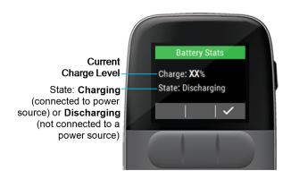
6. Review the *Charge* and *State* of the remote battery and press when finished.
