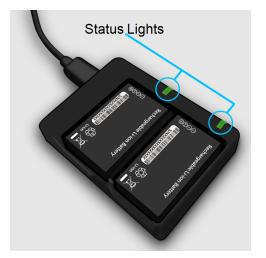
5. If you obtain a pump battery from the remote battery bay, make sure the spare pump battery charging light on the remote, when plugged into AC power, is green. This indicates the pump battery in the remote battery bay is fully charged.
