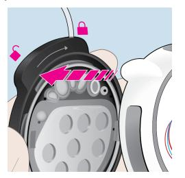
Push down and rotate the pump clockwise to the <u>lock</u> <sup>▲</sup> symbol.
