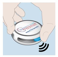
8. If your pump serial number does not show up on screen after a minute, **press and hold** the pump's **blue button** for **10 seconds** to activate pairing mode. This will be confirmed by a single *Ready* beep.
