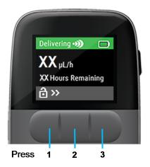
To unlock the remote press the **front buttons** in order from left to right.
