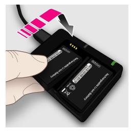
3. If a pump battery is inserted into the remote battery bay, the battery will only charge while the remote is charging.
