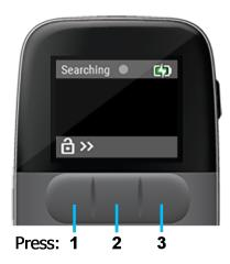
2. Unlock the screen by pressing each **front button** from left to right to unlock the remote screen.
