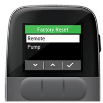
1. Press v to factory reset the remote.
