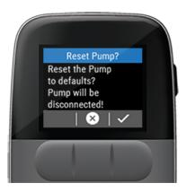
A Reset the Pump to defaults? Pump will be disconnected! message is displayed.
