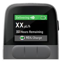
The *Hours Remaining* until the next cassette change is an estimated time based on the fill volume of the cassette and the programmed delivery rate. If the delivery rate is changed after a cassette change, the displayed *Hours Remaining* may no longer be accurate.
