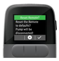
A Reset the Remote to defaults? Pump will be disconnected! message is displayed.
