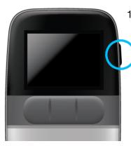
1. Press the **side button** to wake up the remote.
