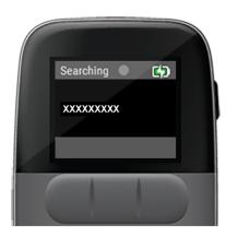
The remote will display *Searching* and the last connected pump serial number until the pump is paired to the remote. See "*Pair to a Spare Pump*" *on page 130.*
