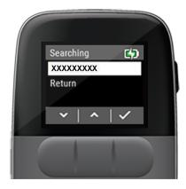
10. When the new pump serial number appears, use the to highlight the new pump serial number and press .
