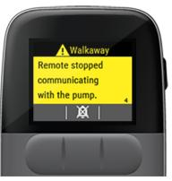
*Walkaway* attention alarm settings are maintained when the system is powered down or loses power.
