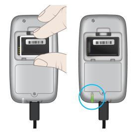
6. Insert the fully charged pump battery into the pump making sure the contacts are aligned.
