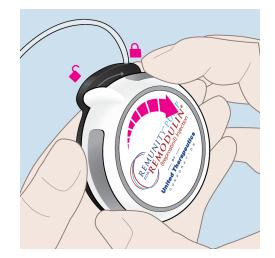
6. *Pump-bump* should align with the infusion set tubing.
