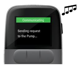
After confirming the new delivery rate, the remote will display a *Sending request to the Pump...* message and you will hear the *Delivering* tone from the pump.
