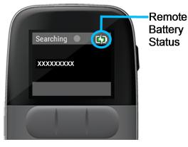
7. When the battery symbol is full green in the status bar, the remote is fully charged.
