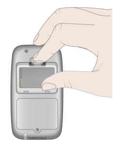
3. Insert a spare rechargeable pump battery into the remote battery bay on the back of the remote making sure to align the contacts.
