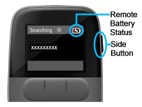
6. Check the status bar for the charging symbol on top of the battery symbol, which indicates that the remote is charging.
