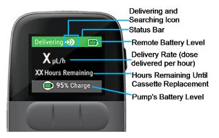
The color of the Status Bar indicates the remote's connection to the pump and the current delivery:
