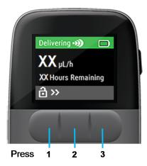
2. Unlock the screen by pressing each front button from left to right.
