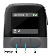
2. Unlock the screen by pressing each front button from left to right to unlock the remote screen.
