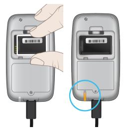
The remote battery bay will charge an inserted pump battery only when the remote is plugged in to charge. A charging spare pump battery is indicated by the amber light on the back of the remote when the remote is powered on.
