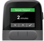
been used and the programmed *Screen Timeout* minutes have passed, you will need to press the **side button** to wake up the remote.
